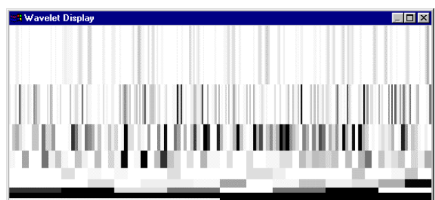
Figure 4: The filter to display the wavelet domain visualizes the multiscale analysis of the wavelet decomposition. The higher the wavelet coefficient in a scale is, the darker the area. The x-axis denotes the time within the audio playback.
